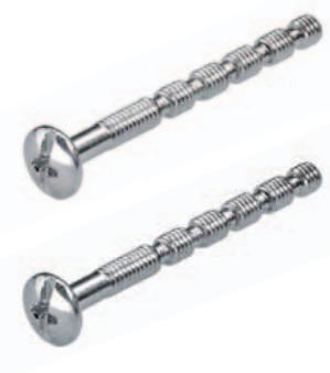
Universal handle cross-slotted fixing screw M4 x 45 mm, can be shortened to 40, 35, 30, 25 or 20 mm Galvanized steel
